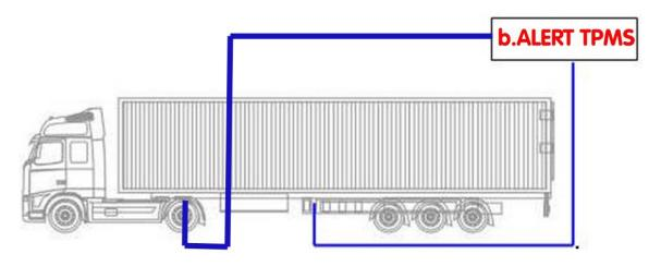
Figure 2 TPMS optimal position
