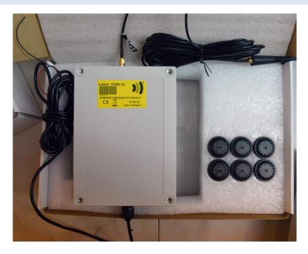
Figure 1 TPMS unit with sensors
