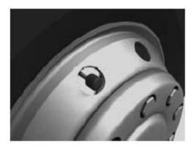
Figure 4 position of tyre sensor
